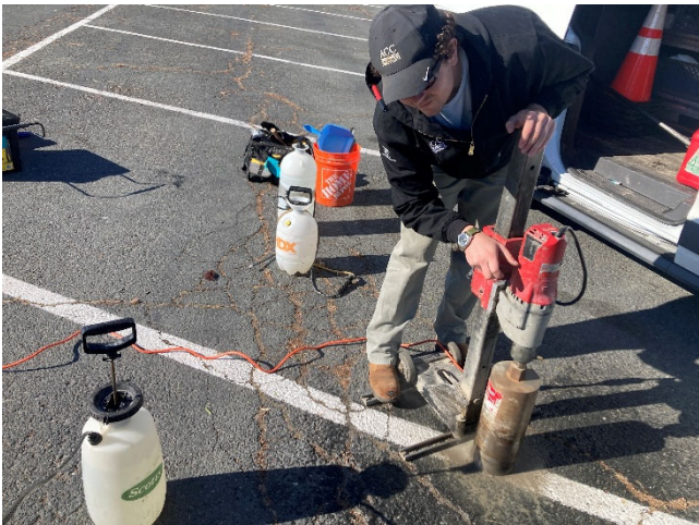
Typical view of ACC using coring machine to core the asphalt paving at the north parking lot.
