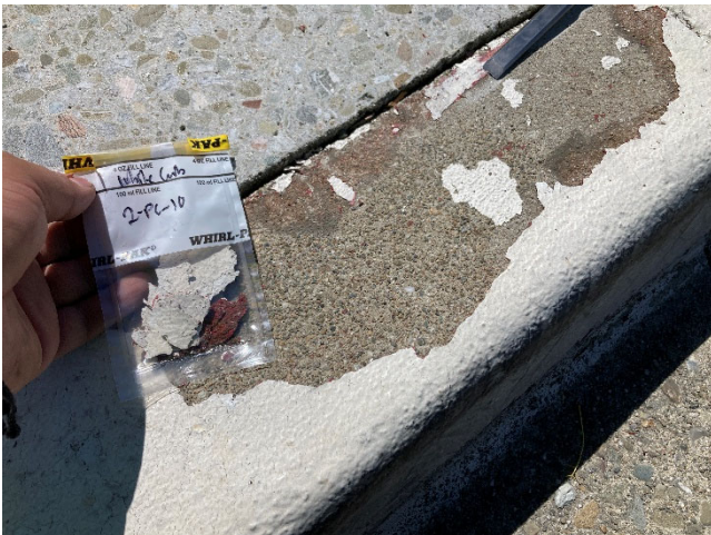
South Parking Lot: View of Sample 2-PC10. The white paint and underlying red paint on concrete curbs were identified to contain lead-containing paint (LCP) at 1,700 ppm.
