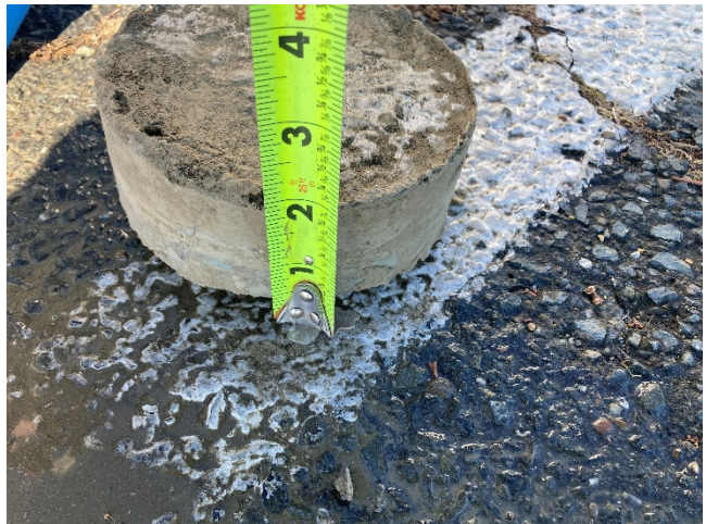
View of asphalt core in the north parking at completion of coring activities (thickness 2"). Sample ID: 2-1-1.
