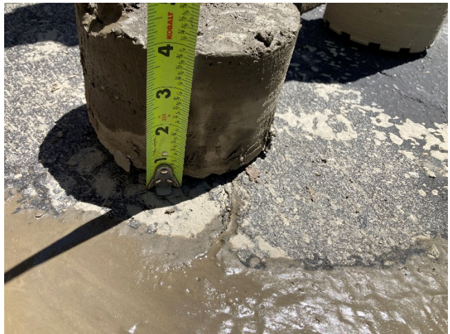
View of asphalt core at portable buildings area at completion of coring activities (thickness 4"). Sample ID: 2-27-2.
