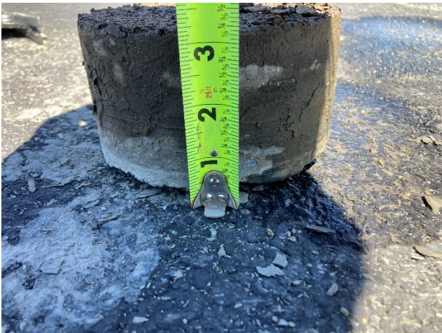
View of asphalt core at portable buildings area at completion of coring activities (thickness 3 1/2"). Sample ID: 2-27-1.
