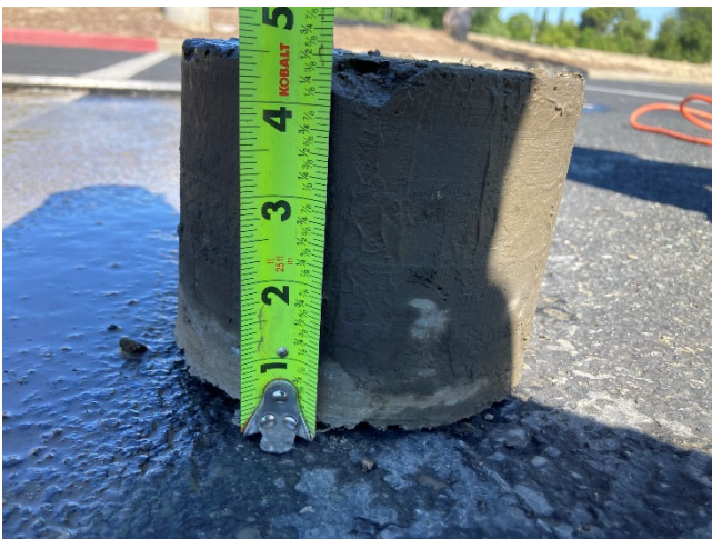
View of asphalt core at the south parking lot at completion of coring activities (thickness 4 1/2"). Sampled ID: 2-9-2.
