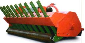
SPF with rakes installed. Rakes float to trace terrain contours.
